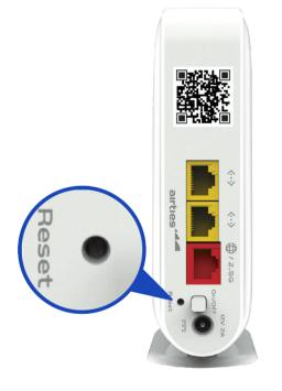
To return the device to factory settings, press down on the reset button (in the small opening on the back shown above) for 5 seconds and release. A metal paperclip (with an extended tip) or strong toothpick are typically good choices for this task. When the reset process is triggered, the LED in the front will "blink rapidly" and the device will reboot to factory settings.
