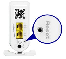
To return the device to factory settings, press down on the reset button (in the small opening on the back shown above) for 5 seconds and release. A metal paperclip (with an extended tip) or strong toothpick are typically good choices for this task. When the reset process is triggered, the LED in the front will "blink rapidly" and the device will reboot to factory settings.
