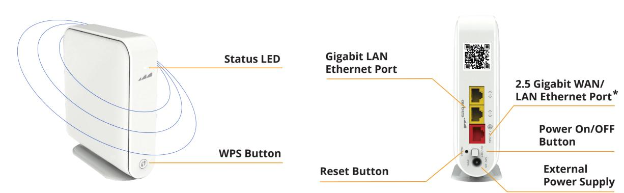
\* Ethernet (Internet) cable from your Internet Service Provider or modem should be plugged into WAN ethernet port of Air 4980 / Air 4985 device.
