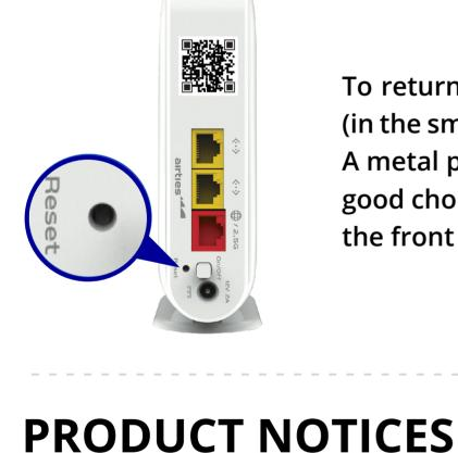
(in the small opening on the back shown above) for 5 seconds and release. A metal paperclip (with an extended tip) or strong toothpick are typically good choices for this task. When the reset process is triggered, the LED in the front will "blink rapidly" and the device will reboot to factory settings.
